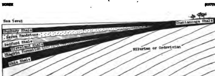
FIG. 1350. — Diagram showing the relation of the black shales to the other formations. The source of the black mud is the land on the south from which it was repeatedly washed into the sea, interfingering with clastics derived from the east. The Berea, Sunbury, and Chattanooga formations are Lower Mississippian, the others Upper Devonian. (Original.)
